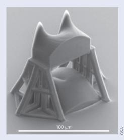
After printing, the structures were rinsed in developer and treated with isopropanol for clean-up. The volumes of the two components (transformer and corrector) are  $60 \times 60 \times 32 \, \mu m^3$  and  $60 \times 30 \times 51.5 \, \mu m^3$ , respectively; the two components were separated by a distance of  $60 \, \mu m$ .
